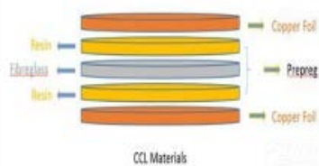
Indicative diagram of layers
